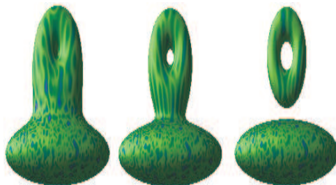
Figure 8: Changing the area of influence and \vartheta . The Z function is defined as a FRep tree, composed of an intersection of a block and a torus. The parameter varies in a similar way as in 6
