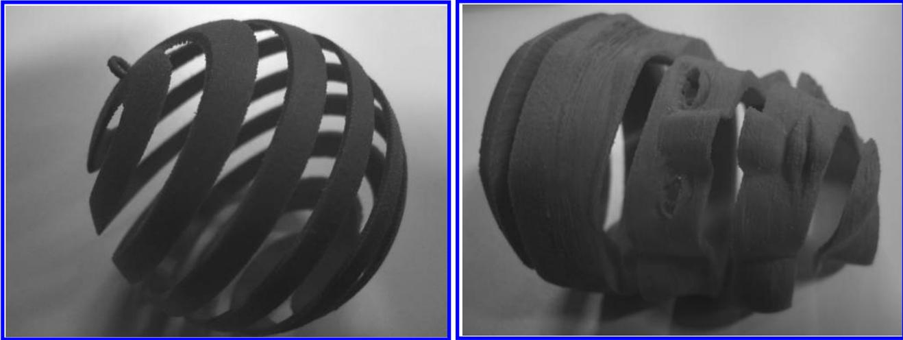
Fig. 7. Physical models printed by FDM Vantage I. (© Alexander Pasko)
