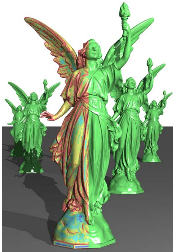
Figure 1: The Stanford Lucy, consisting of 14 million points, is reconstructed as an MPU implicit with a 10^{-4} max-norm approximation accuracy; the left part of the model is colored according to the subdivision level which increases from blue to red. The four models in the back are reconstructed from the point set with increasing approximation error.
